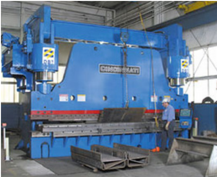
1500-ton PROFORM press brake brings built-to-last structural strength, enhanced precision, Windows touchscreen ease of setup and programming to flexible production by DBT America of plate components up to 2" thick for "made to order" mining equipment.
