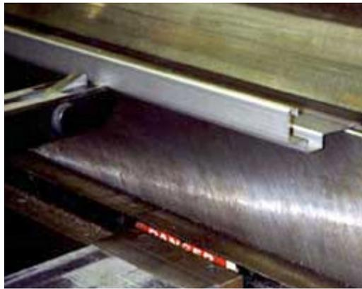
*CNC frontgaging on CINCINNATI Autoform press brakes halves setup time, holds +/-0.015" precision on commercial door system components.*
