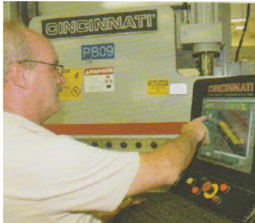
*A Midland press brake operator preps a file on a CINCINNATI Autoform press brake. Midland averaged 35 full-sized, fully functioning prototypes per week in 2010. Interface between software (Solidworks) and machines enables Midland to receive a design file, send the flat files to the laser, send the formed files to the press brake and have a prototype the same day.*
