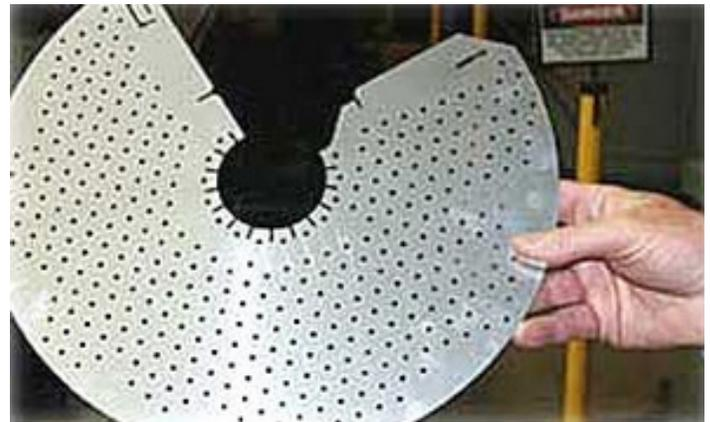
Herstine. The most common materials are 1/4” to 1” thick A572-50 or ASTM A514 steel, but certain products require AR400 and AR450 plate ranging from 3/4” to 2”.
