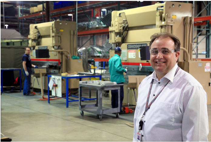
Dan Sizemore is plant manager for Humvee up-armor production at BAE Systems in Cincinnati. The plant is organized for 2417 cellular production. Flow through processing starts with cutting part shapes out of plate. Components are next bent on CINCINNATI press brakes and then sent to robot welding.
