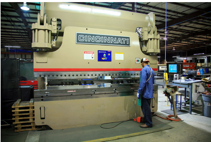
Standardizing on CINCINNATI press brakes allows interchangeable dies, programs, and operators, simplifies training and maintenance, and enables maximum flexibility in scheduling. The company has 11 CINCINNATI press brakes bending armor parts - eight for Humvee up-armor kits, three for the Caiman MRAP program.
