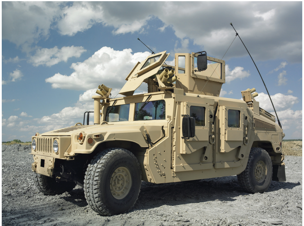
Up-armored Humvee features under-body armor cladding, thicker armored doors, and ballistic glass. Eighty Up-Armor kits produced by BAE in Cincinnati ship daily to AM General's Humvee plant in Mishawaka, Indiana, for truck assembly.
