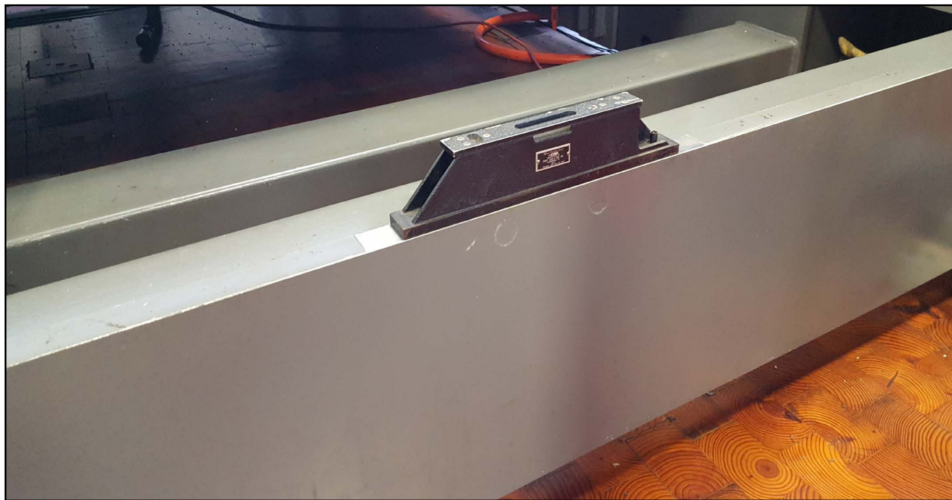
FIGURE 2-4 Cross leveling (Preliminary)
