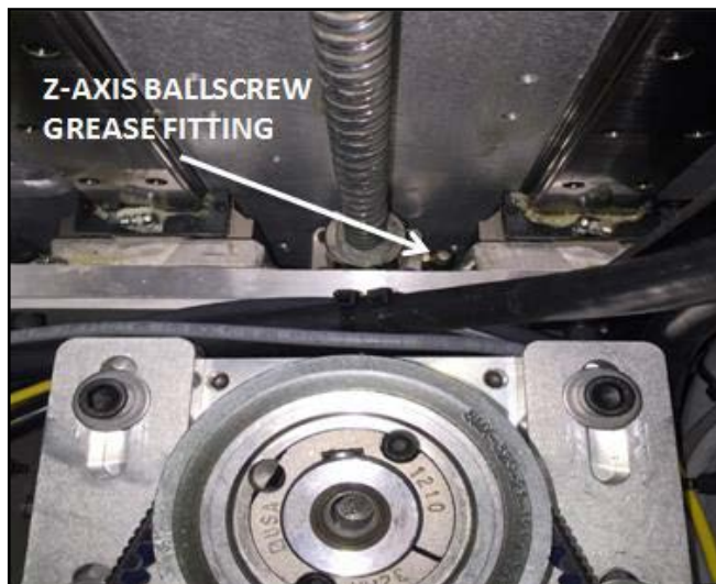
FIGURE 9-4: Ballscrew Lube Point
