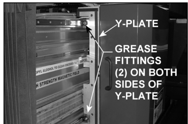
FIGURE 9-2: Y-Axis Linear Bearing Grease fittings (Do not over-grease)
