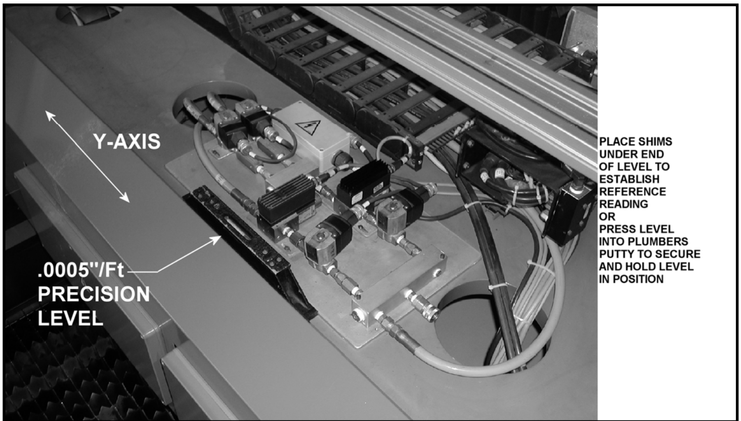
FIGURE 2-6 Final leveling with precision level
