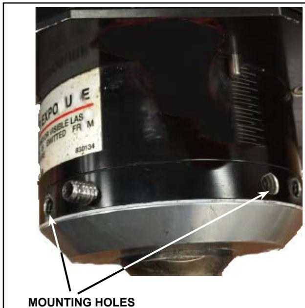
**FIGURE 3: Mounting Location**
