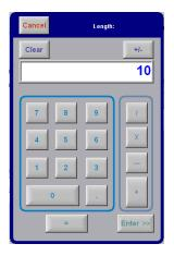
When the user touches a numeric entry field, the Pop-up Calculator will automatically open. To enter a number, press the buttons on the Pop-up Calculator. To transfer the displayed number into the numeric entry field, press the "Enter >>" button.
