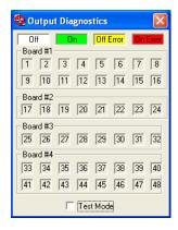
This dialog shows the status of up to 32 digital outputs. Green indicates that an output is on; white indicates that an output is off; yellow indicates that an output is "On Error"; red indicates that an output is "On Error", and gray means that an output is not installed.
