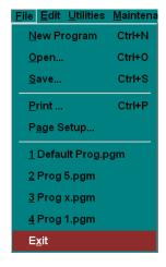
The *File* menu contains commands for loading, saving, and printing files as well as exiting the Shear Control application.
