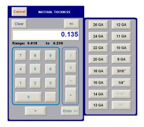
When the View Units are "English" and the thickness corresponds to one of the buttons, the thickness is also displayed with the gauge number or inch fraction designation in a label next to the "Material Thickness" field. The label text is the same as the text on the calculator add-on button.
