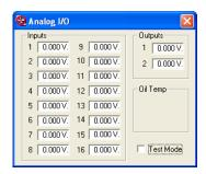
This diagnostic dialog shows the values of the 16 analog inputs (in Volts), the 2 analog outputs (in Volts), and the oil temperature (in °F). Oil temperature(s) will only be displayed if the machine is equipped with an oil temperature sensor.
