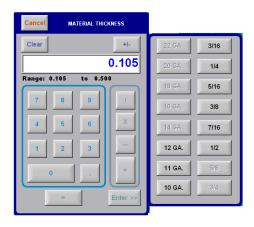
If View Units are "English" and the Thickness is selected with one of the add-on buttons, the software also displays the button text as a label next to the "Material Thickness" field.
