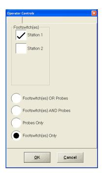
**Note:** If Cycle Status is **Ready**, then changing the active **Operator Station** settings (by pressing the "OK" button) will change Cycle Status to **Idle**.
