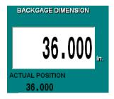
The "Dimension" field indicates the commanded position. To alert the operator when the gage is moving to the next commanded position, the Run / Edit page displays the actual position under the command value. The Run / Edit page always displays the actual position in decimal units.
