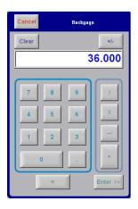
The Pop-up Calculator may also be invoked by pressing the "TOUCHCALC" button in the Toolbar. This opens a standalone version of the Pop-up Calculator for quick calculations. There is no "Enter >>" button because the value is not associated with any particular field.
