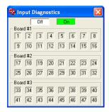
This dialog shows the status of the 48 digital inputs. Green indicates that an input is on and white indicates that an input is off.
