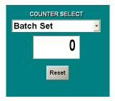
6. Run the program. The display begins with *Batch Count* equal to the *Batch Set* value. The control reduces the count by one every time the program finishes. When the *Batch Count* display reaches zero, the control disables the shear and displays the *Batch complete* message:
