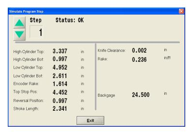
The Step up / down arrows allow the user to display the values for each program Step. The 'Status' line indicates any errors generated by the displayed program Step.
