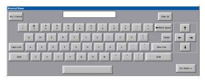
Selecting an alphanumeric entry field will open the Pop-up Keyboard. An example of an alphanumeric entry field is the "SETUP NOTES" field on the Spreadsheet page.
