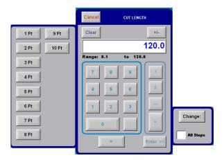
If View Units are 'English' and *Cut Length* is selected with one of the add-on buttons, the software also displays the button text as a label next to the "Cut Length" field.
