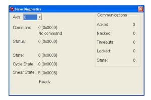
The left side of this dialog is used by CINCINNATI INCORPORATED personnel. The right side shows the status of the serial communications link between the Shear Control and the Slave computer. The number of "Acked" packets should increase several times a second. Excessive numbers of "Nacked" packets or time-outs may indicate a problem with the serial communications cable.
