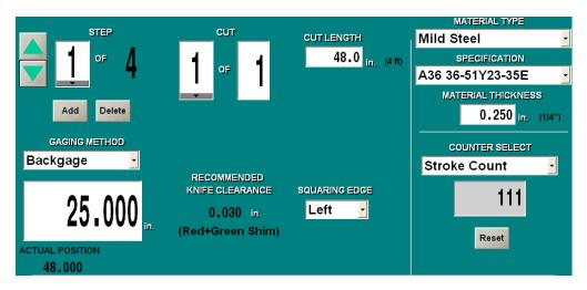
The main area of the Run / Edit screen displays settings related to the currently open program file. The settings are displayed in editable fields and informational fields. For example, in the figure above this paragraph, "CUT LENGTH" is an editable field and "KNIFE CLEARANCE" is an informational field.
