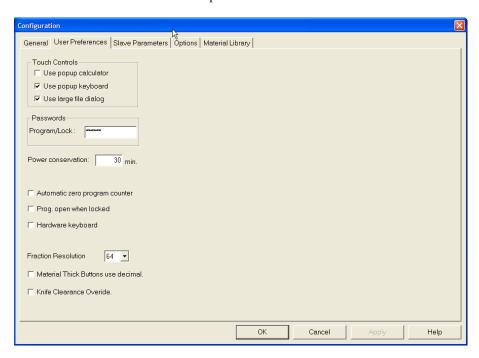
The **TOUCH CONTROLS** section includes check boxes to specify whether the application will use the Pop-up Calculator or keyboard.
