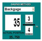
Changing the Units selection to **English** | **Fraction** will cause the gage dimension to be rounded off to the nearest fraction of an inch specified in Configuration (User Preferences page, *Fraction Resolution* setting). Any fractional part is displayed in simplest form.
