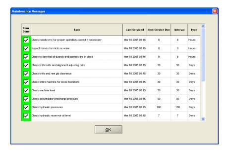
This dialog displays the list of scheduled or completed maintenance tasks and allows the user to acknowledge task completion. The user can also create up to ten user-defined tasks and specify the scheduled interval for each.
