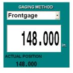
To edit the gage position command, select the field and type a new value in the Pop-up Calculator. If the shear has both gages, the Pop-up Calculator includes an add-on with buttons to select the gage. If a different gage is selected with the add-on button, closing the calculator will change the 'GAGING METHOD' selection on the Run Edit page.
