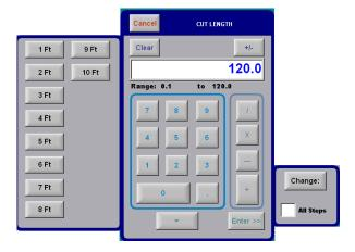
When the View Units are "English" and the *Cut Length* rounded to the nearest inch is a multiple of 12, then the length is also displayed in feet units as a label next to the "Cut Length" field.
