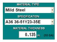
**Note:** For a model 135 shear, all programs use the same rake and knife clearance; the Material Settings only notify the operator which material and thickness to load for the selected program.
