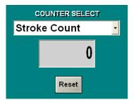
The list box selects the function of the display: "Stroke Count", "Batch Set", "Batch Count", or "Program Count". For more information, see **COUNTER SELECT** in the **RUN / EDIT PAGE** section of this manual.
