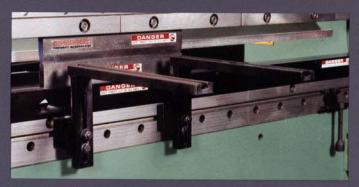
CINCINNATI Work Support Brackets permit increased efficiency in handling material at the front or rear of the press brake. Horizontal support can be 24 inches, 36 inches, or 48 inches depending on the application.
