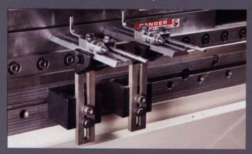
All gages can be set for forming wide or narrow sheets either upward or downward. They can also be used as an adjustable two-step gage. CINCINNATI Standard Gages are available with or without micrometer adjustment to the gage rod.
