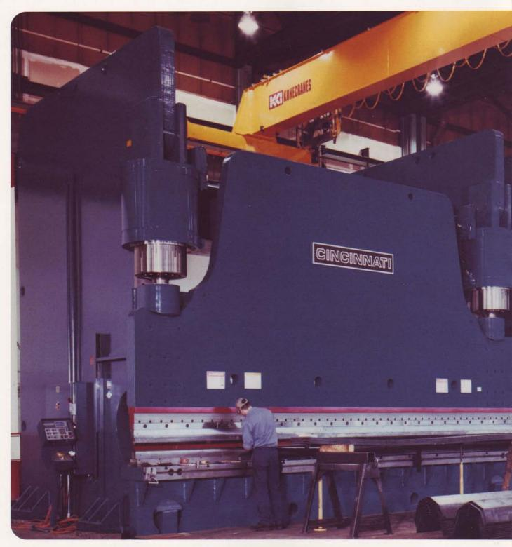
Tandem CINCINNATI 2000 ton Form Master Hydraulic Press Brakes having a combined length of 50 feet enables this fabricator to apply up to 4000 tons of force in the production of chassis frames and rails for fire trucks, motor homes, custom trucks and telescopic conveyor systems.
