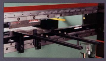
CINCINNATI Heavy Duty Gages with massive stops are particularly recommended for use in plate shops where very rugged construction is necessary.
