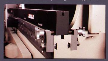
CINCINNATI Die Aligners enable filler blocks and keyless dies to be aligned on the press brake bed. These items are designed to fit a dovetail slot in the bed and are furnished in a set of six.
