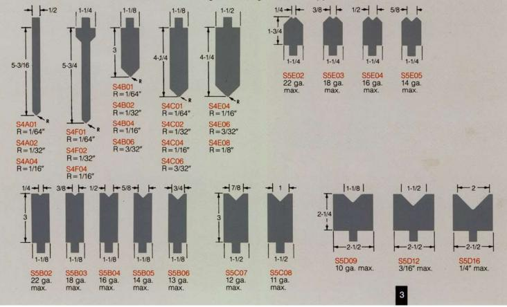
Gooseneck dies are used for making channels or special shapes with which a straight sided die would interfere. Deeper "throat" beyond the die centerline increases width of return flange but reduces die capacity. Interference can be checked using a gooseneck die template which can be requested from CINCINNATI.
