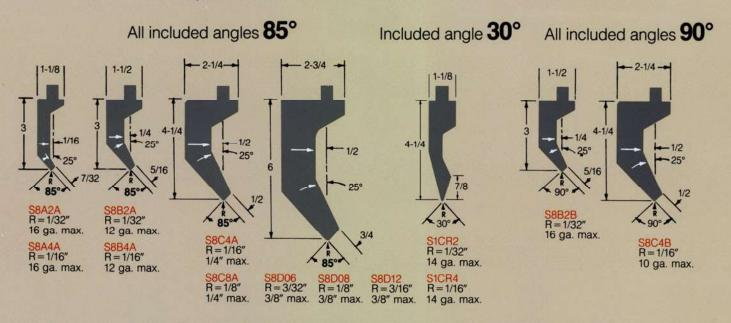
If parts are to be formed with "air bend" dies on a press brake with controls that use mathematical models (i.e. AUTOFORM®) to determine ram reversal positions, the dies must be cut to a 75 degree or less angle to compensate for all possible material springback. In some cases, 30 degree dies can be selected to obtain true air bending of 90 degree angles.
