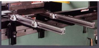
CINCINNATI Adjustable Flip Gages provide multiple gaging positions with complete flexibility in vertical and horizontal positioning. Disappearing gage assemblies with either 5/16" or 5/8" rise are located on either side of heavy duty gage bars. Scales graduated in sixteenths are mounted flush on each side of the heavy duty gage bars. Any number of stops may be used.
